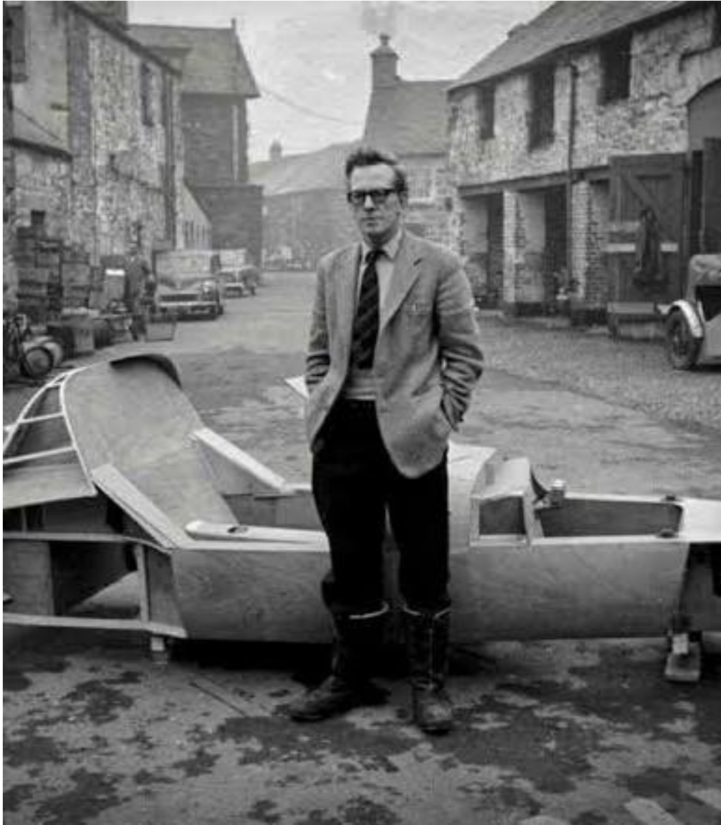
Frank in his 'Wellies' posing with one of his radical monocoque plywood race cars.
