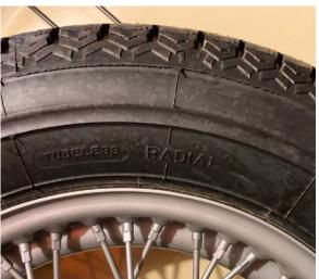
Here's a side by side comparison; bias ply tire on the left, radial on the right. Note the "crew cut" appearance of the tread on the bias ply and the rounded tread on the radial. The Dunlop tire on the left is a 69 year old original tire supplied on our 1955 MG TF 1500. I'll bet it is still filled with air from Abingdon!
