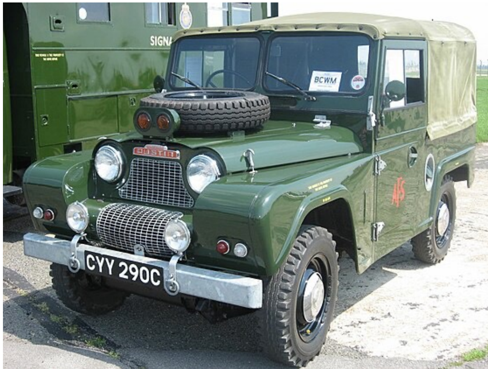
This is a short wheelbase version of the Gipsy with canvas top erected. Photo courtesy of Wikipedia.
