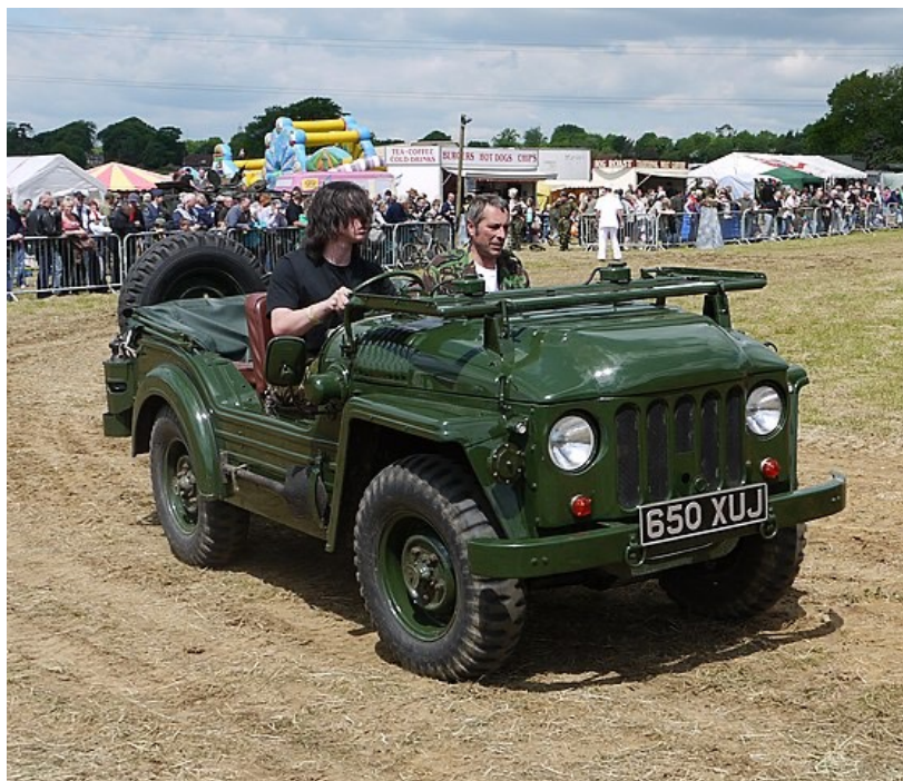
The Austin Champ resembled the American Jeep but was far more complex, difficult to maintain with its four wheel independent suspension and Rolls-Royce sourced engine, and too expensive to continue to serve in the British Armed Forces. Photo courtesy Wikipedia.
