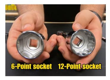
The 6-point socket walls are thicker than the 12-point and the walls are slightly convex curved between the points. (Western Equip photo)
