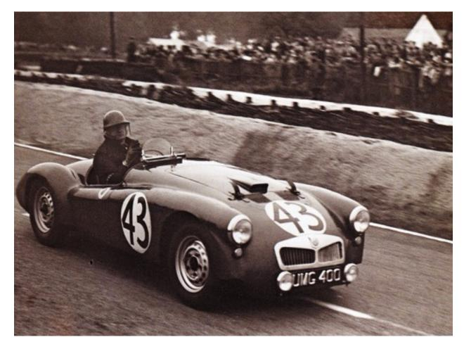
UMG 400 or project number EX176, was built for the 1951 Le Mans 24 hour race and showed the way ahead for the MGA as did the faired in headlights for the TF that came along three years later. The streamlined body was a big improvement over the TD on which it sat but unfortunately the narrow TD chassis forced the driver to be perched high above the cowl. A new chassis for the MGA with wider side rails allowed the driver to sit lower in the car and out of the wind stream.
