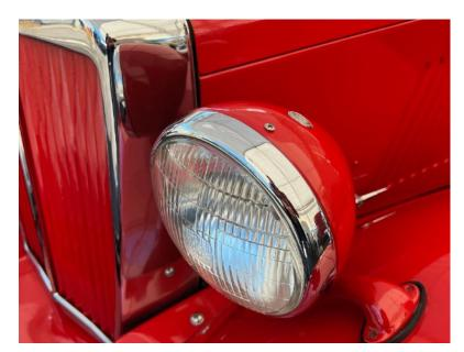
As production rolled on all TDs received chrome plated headlamp buckets until stocks were depleted. At that point reject buckets with stamped orifices were painted body color, received chromed "King of the Road medallions" and were sent to the assembly line.
