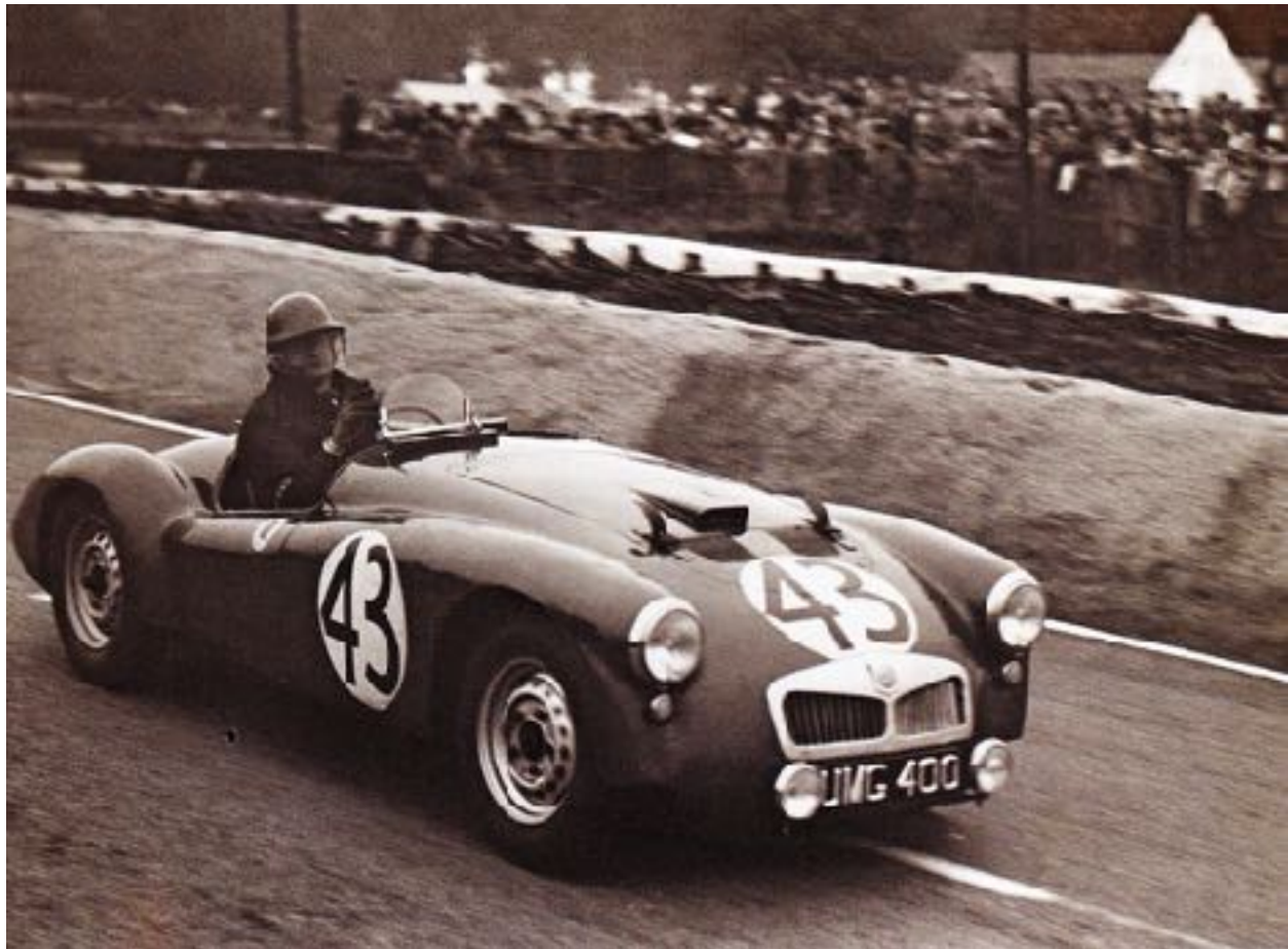
UMG 400 on the track at the 1951 Le Mans 24 Hour race. Notice how high up the driver is sitting. A revised chassis design fixed the problem.
